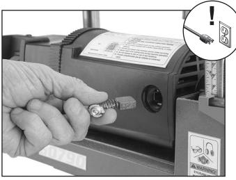
**Figure 31.** Brush holder location. A second brush is located on other side of motor.
